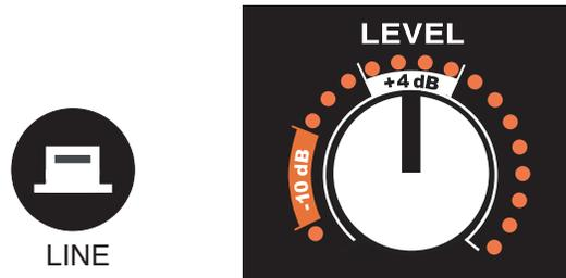
When a microphone, instrument or other consumer product is connected to the system, first ensure that the “LEVEL” control is at its minimum, anti-clockwise, OFF position. Then select the “Mic” input sensitivity and slowly increase the level. If the “overload” LED illuminates you should back the level down again. If the “overload” LED illuminates and the “LEVEL” control is barely cracked open then you should try selecting the “LINE” input sensitivity range.
