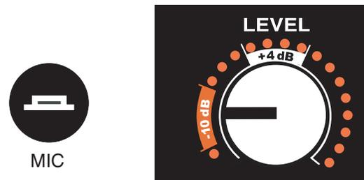
**WARNING: SELECTING THE “MIC” POSITION WITH THE LEVEL CONTROL IN ANY POSITION OTHER THAN THE “OFF” POSITION MAY RESULT IN EXTREMELY HIGH SPLs.**
